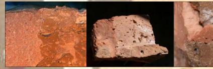
Sample of Ctesiphon brick jointed and substituted with geopolymer. Microscopy points out geopolymer-brick edge.
