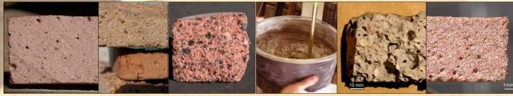
Examples of geopolymer composites with various properties and appearance resembling Ctesiphon bricks
